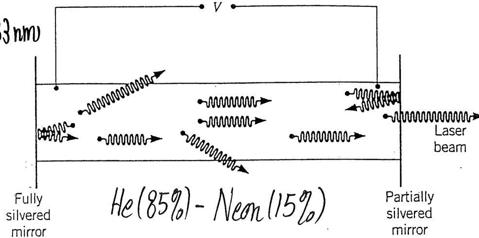
Schematic diagram of a He-Ne laser.
